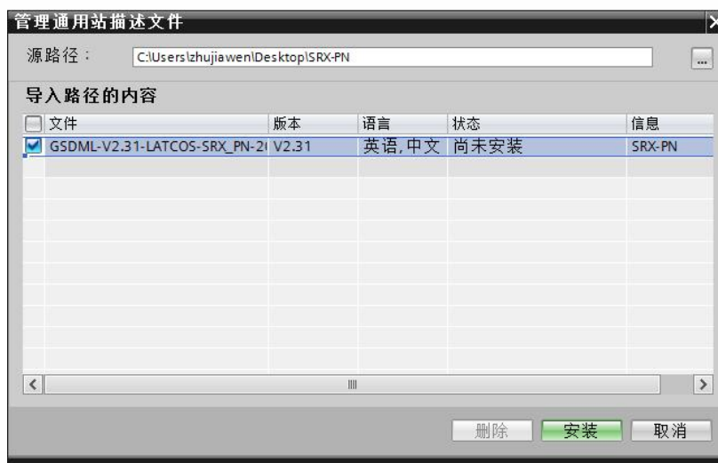
Figure 6-3 GSD Installation Window
